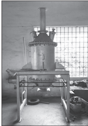
Fig. 2 - Furnace used to obtain the ash and to burn the bricks
